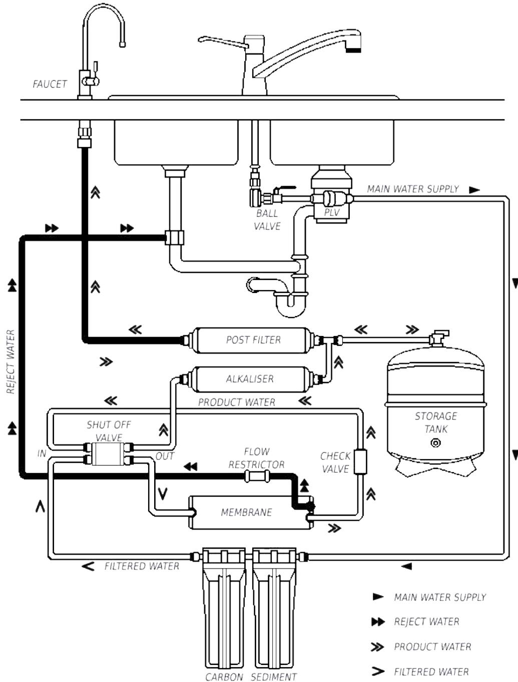
**\*\* Plumber to connect reject line to the sewer in accordance with AS/NZS3500.2 regulations \*\***
